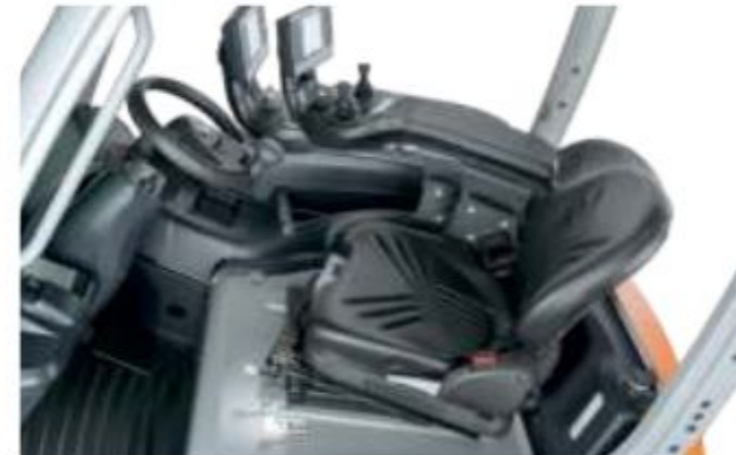
Swivel seat for comfortable reversing
