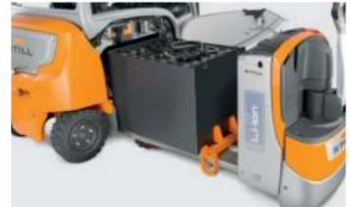
Battery change with electric pallet truck
