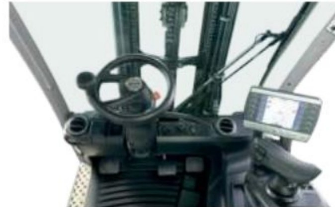
Workspace with display and control units, Joystick 4Plus and heating
