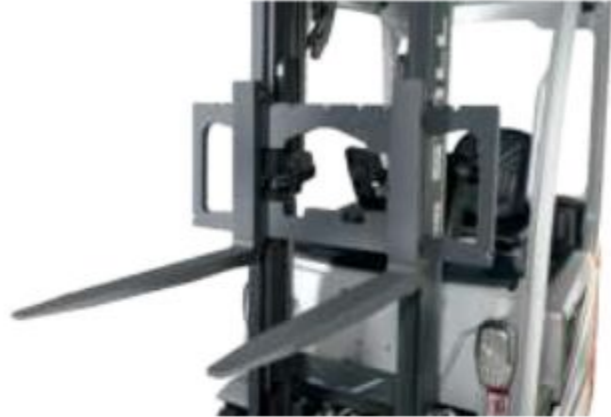
Optimal view of fork tips when loading HCVs
