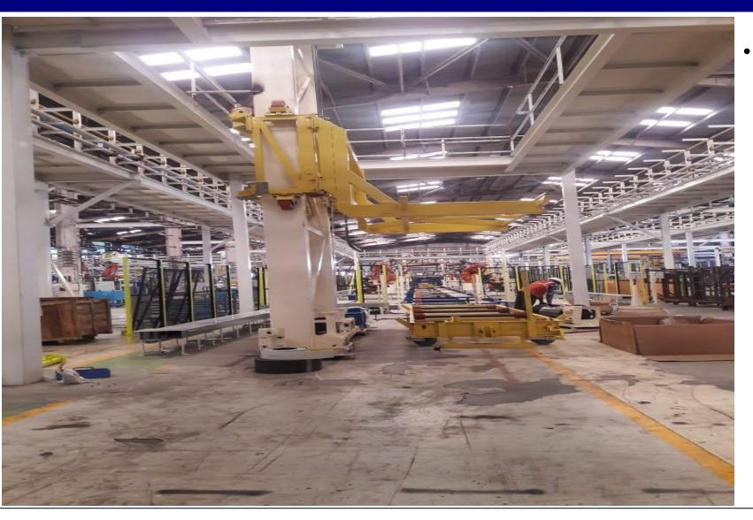
Transfer of Car body from Floor level to overhead Transfer system.
