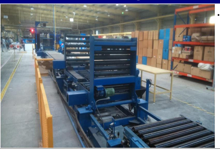
The Equipment is used to tilt the component so the operator can assemble the equipment in a comfortable position.
